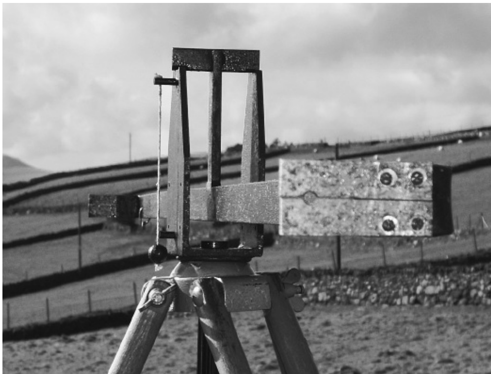
FIGURE 5.16 Reconstructed libra, detail. Photograph by the author.
