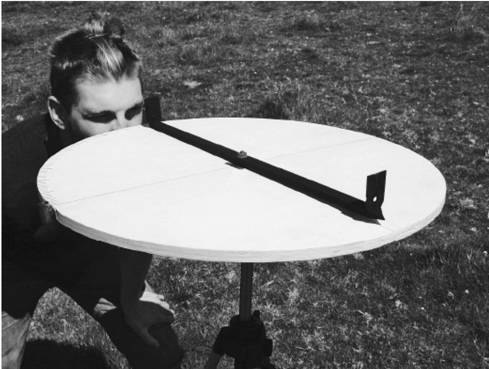
FIGURE 5.2 Reconstructed standard dioptra in horizontal mode. Photograph by the author.
